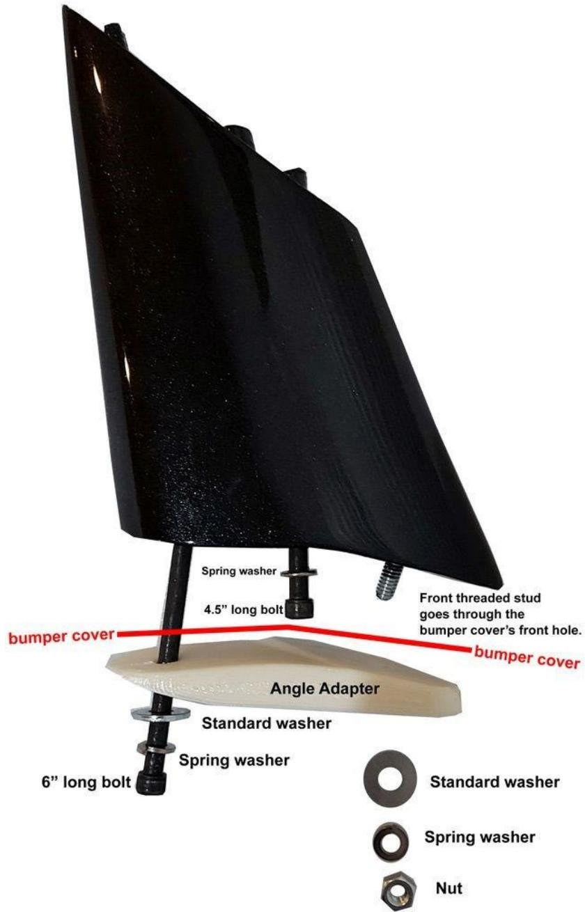
NOTE: Standard washer, Spring washer and Nut illustrated above secures the threaded stud from underneath the adapter.
